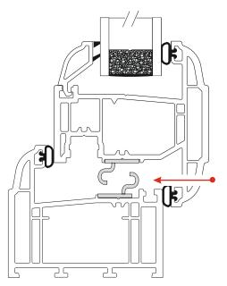
**STAY GUARD ELITE SG036** on outer frame and sash for types of stay to include Egress/Easy Clean
